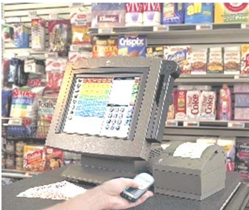
Figure 10: Mobile Local Payment at POS with PIN-code entry through the mobile device
